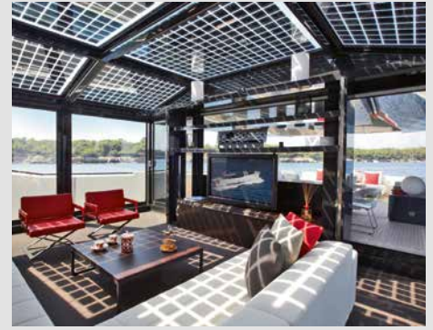
GEWE-sol® PV as a shading element
